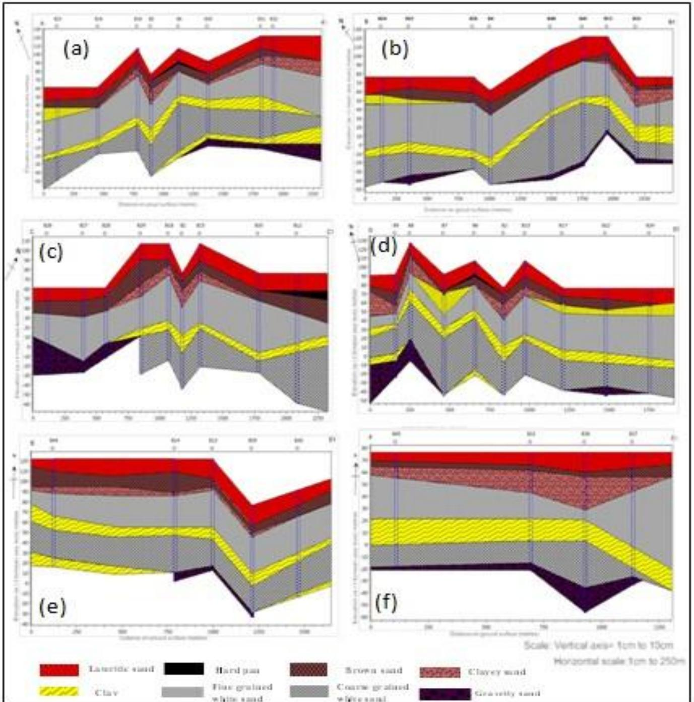
Fig.5: Panel diagrams along the section (a) A-A1; (b) B-B1; (c) C-C1; (d) D-D1; (e) E-E1 and (f) F-F1.
