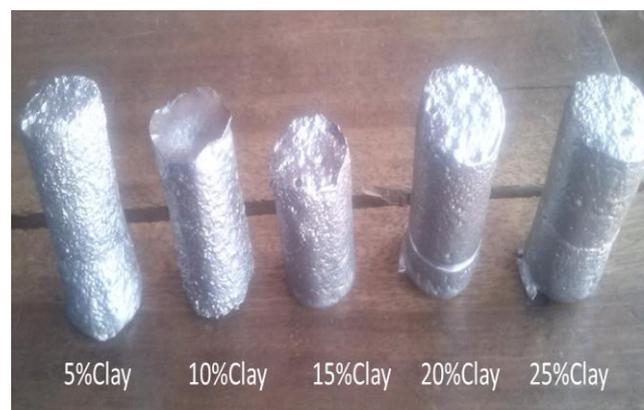
Plate 2: Surface appearance of Aluminum ingots casted from the blended sand
