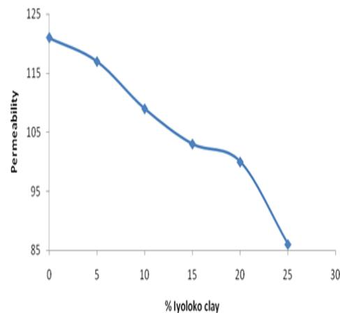
Figure 3, Variation of Permeability with % of Iyoloko clay
