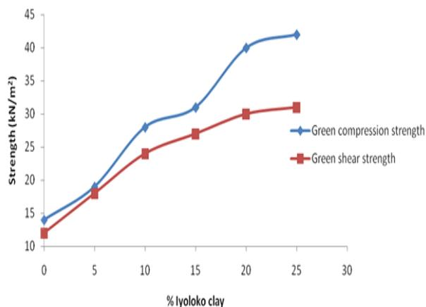
Figure 6, Variation of Green Strength with % of Iyoloko clay
