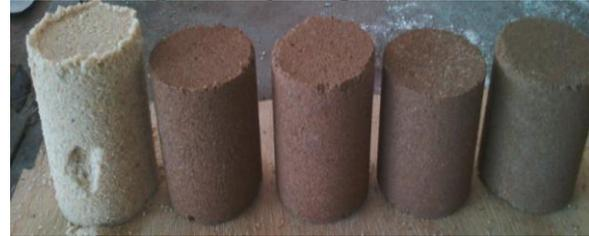
Plate 1: Standard test sample for the Green sand properties
