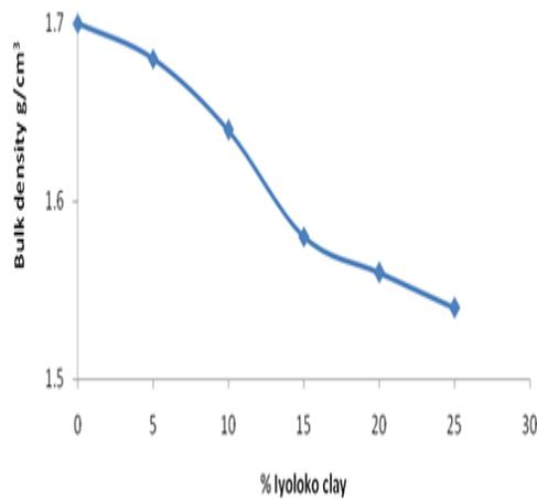
Figure 2, Variation of Bulk Density with % of Iyoloko clay
