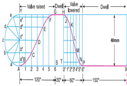
Fig 6: Displacement of CAM
