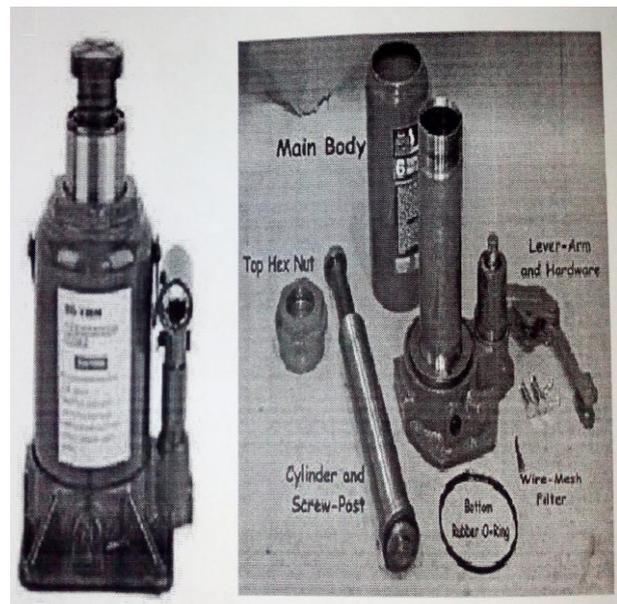
Fig 3: Bottle Hydraulic Jack (Exploded)
